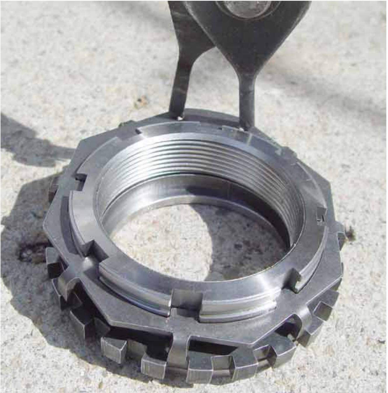
Now comes the snap ring that holds the "spider" pressed tight into the "star". Notice there are two different snap ring slots? This makes it nice because you can install the nut either direction and you can still assemble everything...another good idea by the manufacturer.
