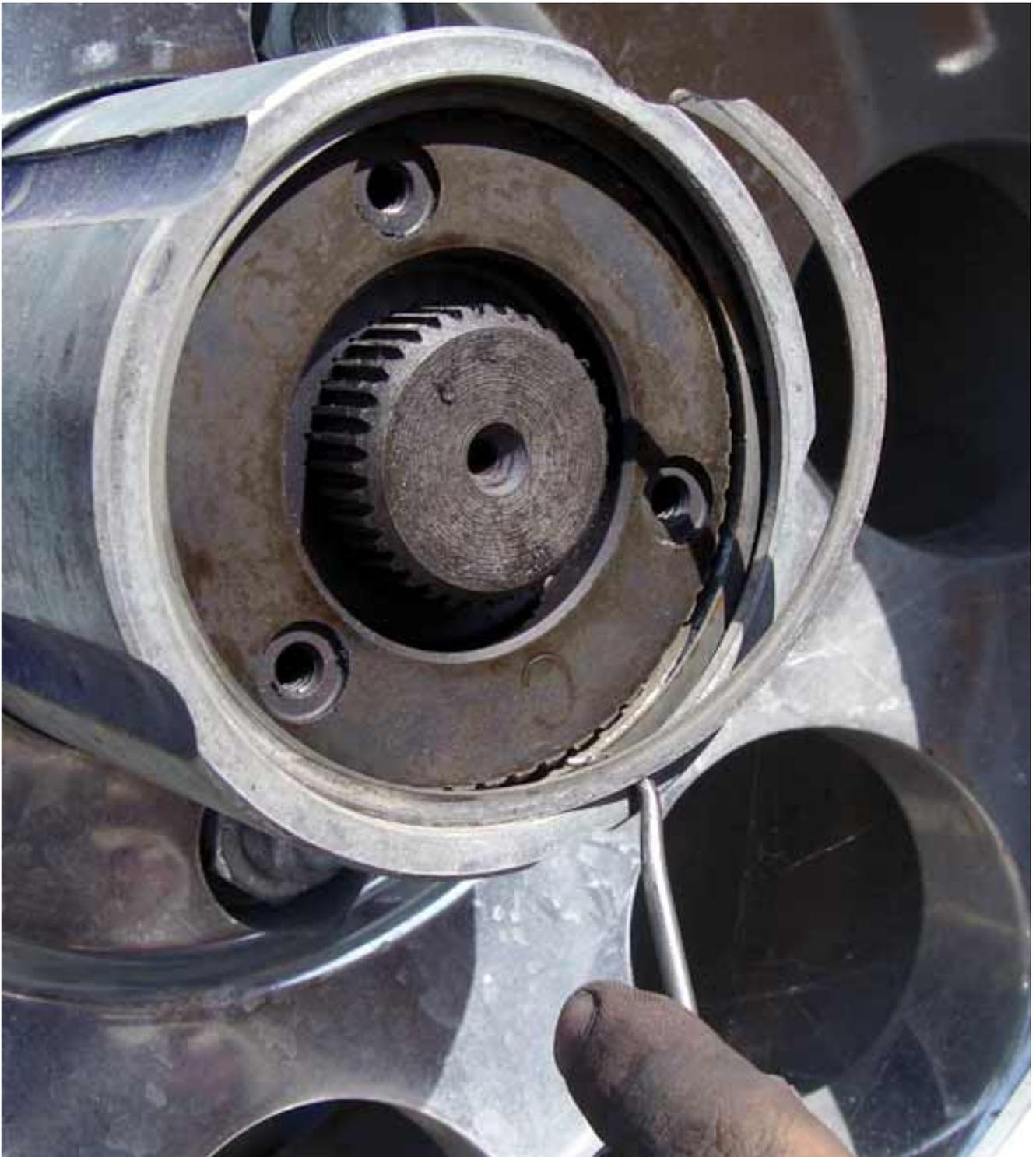
Using a bolt taken from the flange cover we just removed, Mike screws it in a few turns to create a handle to pull the slug out with. If it doesn't come easily, Mike can just spin the wheel to relieve possible tension on the axle or flange splines. Note the dirt on the outer edge of the outer flange splines???.someone's in trouble for installing a dirty flange during a speedy swap at a recent event ;-)
