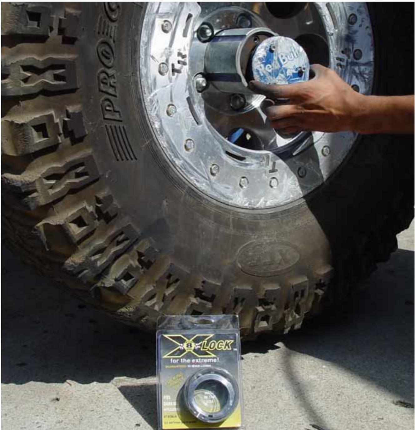
Then Mike used a small pick to remove the spiral clip that holds the actual drive "slug" in place. This is a PolyPerformance Drive Flange by the way...other brands may remove/install differently.
