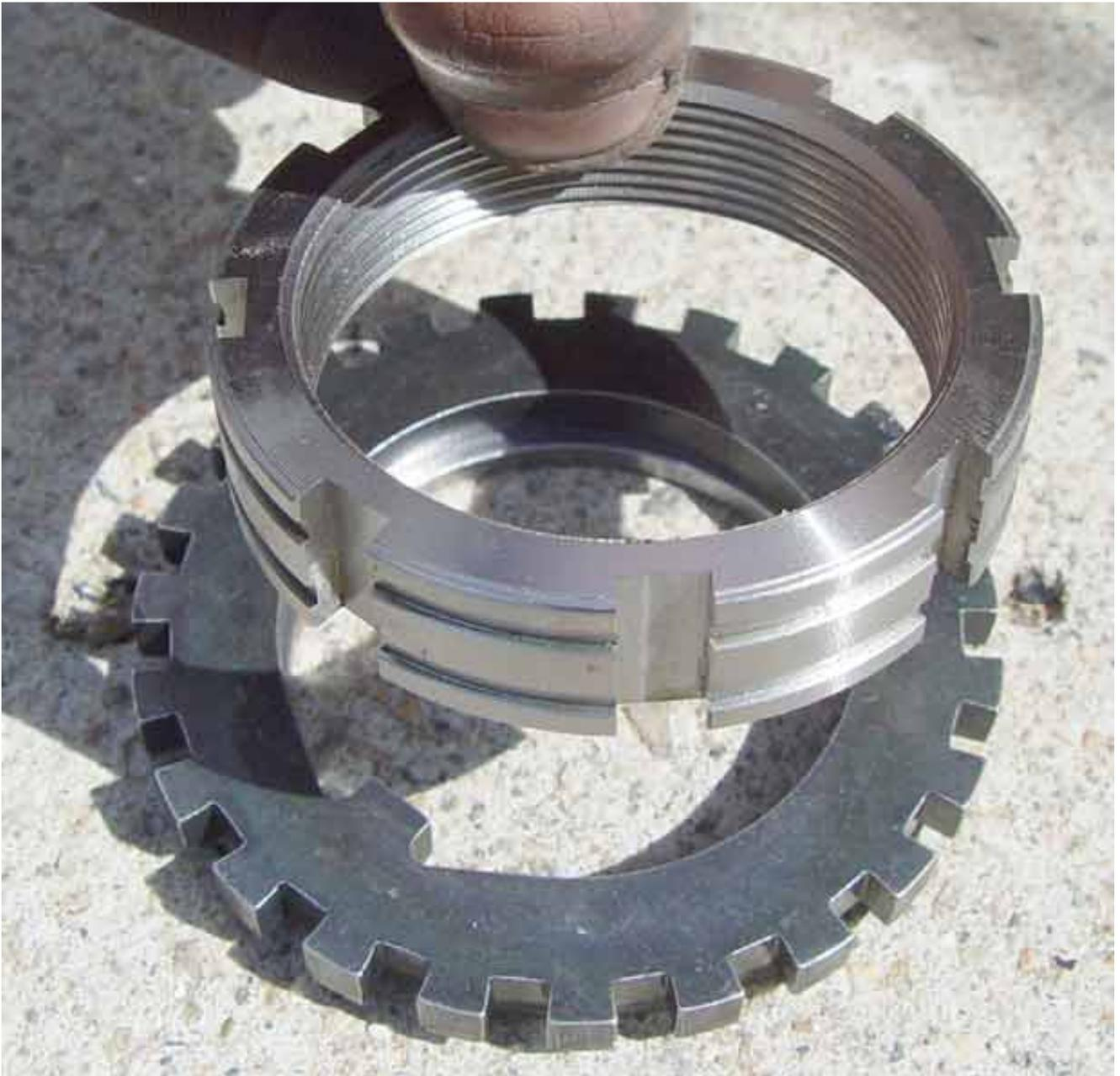
Next comes the locking assembly that I'll call the "spider". It can be installed with a set of snap ring pliers as there are two holes simply for holding it that way. You don't actually "spring" them with the snap ring pliers, you only hold them. That was a great idea as installing and pulling those Spicer washers is a hassle if you don't have tiny fingers. Indexing the Stage 8 version is a cakewalk.
