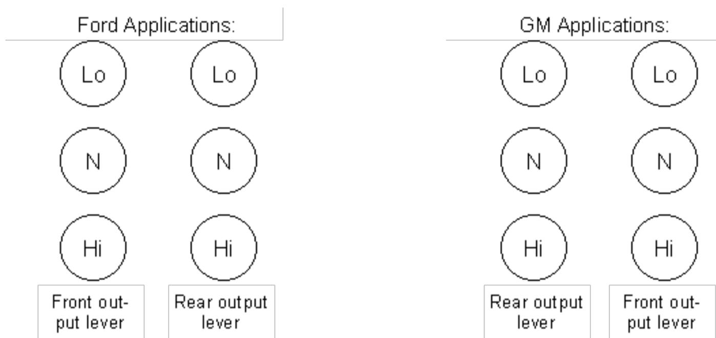
There are some common misconceptions about the way the shifters on a NP205 work. The biggest is that there is a "4wd lever" and a "hi-lo" lever. This is false. The 205 has one shift rail that controls the front output shaft and one that controls the rear output shaft. With ORD shifters, you have 3 positions on each shifter stick as illustrated above.
